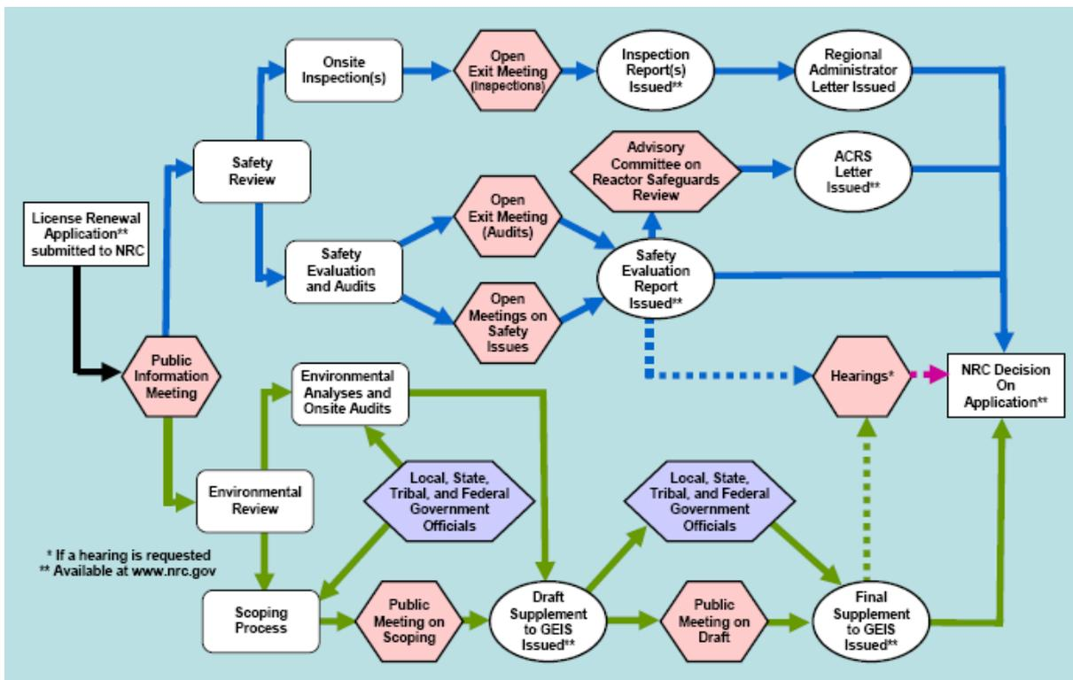
Figure 2. NRC LR and SLR Review Process [3]
